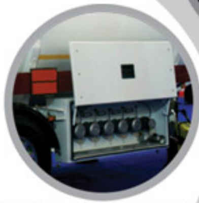
Discharging Box and Valves
